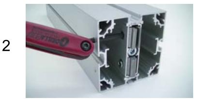
Turn the hex wrench clockwise to open the lock and secure in the groove.
