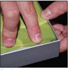
Step 2 Repeat Step 1 for opposite corner C, then insert corner B, followed by corner corner D, to complete the installation of the corners.
