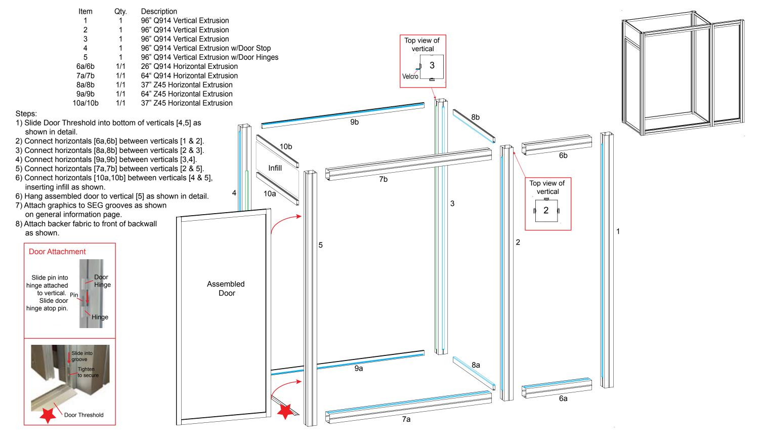
WHEN DISASSEMBLING ALUMINUM EXTRUSION, TIGHTEN ALL SETSCREWS AND LOCKS TO PREVENT LOSS DURING SHIPPING
