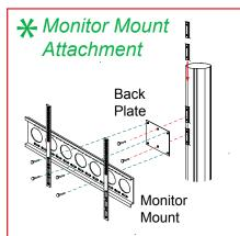
Slide mounting connector pieces into groove of extrusion. Tighten setscrew to secure in place.
