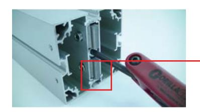
Turn the set screw clockwise to move the lock back into the extrusion, counter-clockwise to move the lock outward.
