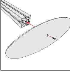
**Base Plate & Extrusion Connection**
