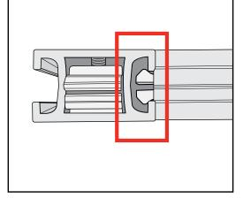
**Extrusion & Lock Connection**
