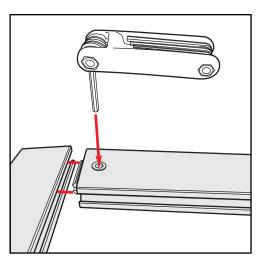
**Extrusion & Lock Connection**
