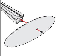
**Base Plate & Extrusion Connection**
