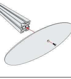
Base Plate & Extrusion Connection
