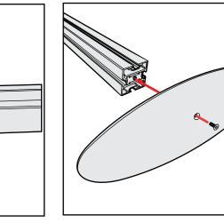
Base Plate & Extrusion Connection
