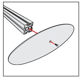
Base Plate & Extrusion Connection
