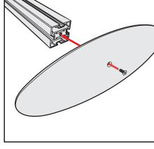
Base Plate & Extrusion Connection
