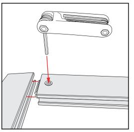
Extrusion & Lock Connection
