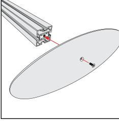
Base Plate & Extrusion Connection
