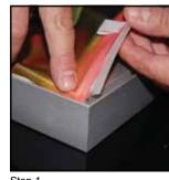
Insert corner A Turn edge of graphic so silicon welt is perpendicular to face of graphic. Insert narrow side of welt with fabric to outside into the channel.
