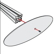
Base Plate & Extrusion Connection
