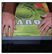
Step 3 Once all corners are inserted, press one silicon edge into channel from corners and work toward the center. Make sure welt is fully inserted into channel. Continue until all sides are done. Smooth out edges of graphic.
