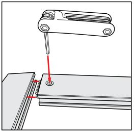
Extrusion & Lock Connection
