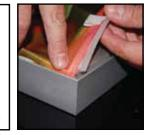
Step 1 Step 2 Insert corner A. Turn edge of graphic so silicon welt is perpendicular to face of graphic. Insert narrow side of welt with fabric to outside into the channel. Repeat for other side of this corner.
