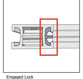
**Base Plate & Extrusion Connection**
